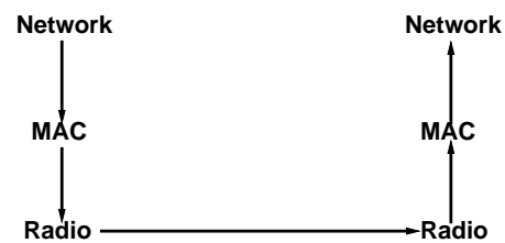
Figure 3.2: The protocol layer structure for wired and wireless transmission.
