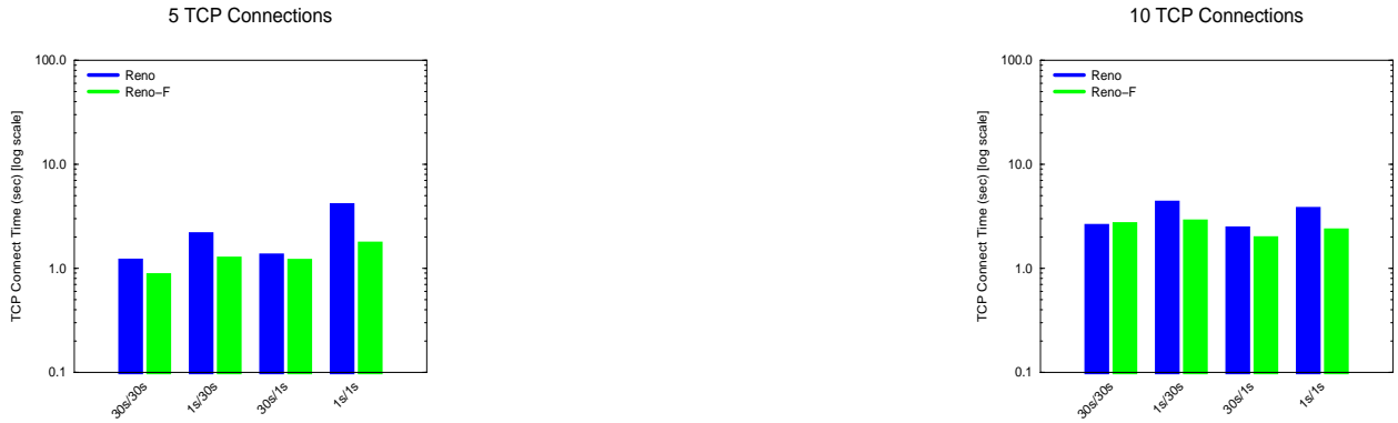
Figure B.11: Connect times for ADV for 5 and 10 TCP connections with a 200 Kbps background load from 10 CBR sources.
