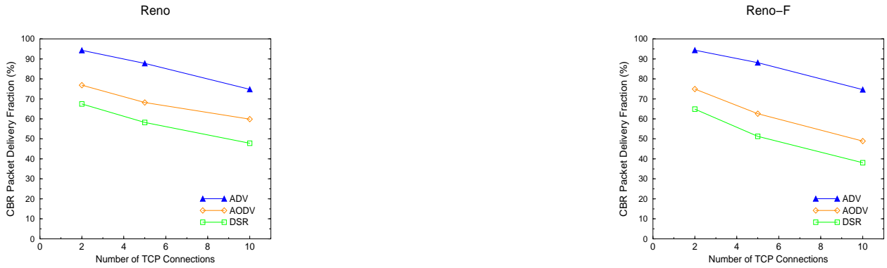
Figure B.10: CBR packet delivery fractions for TCP Reno and Reno-F with a 100 Kbps background load from 40 CBR connections.
